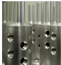
What sounds simple actually poses huge challenges in terms of production technology. Aside from the fact that thousands of amps of current are in contact with the metal parts, the various different materials used in the area of energy distribution also poses a challenge. «We usually have the components plated in silver or tin to prevent corrosion,» explains Sefag product manager Daniel Bieri.
